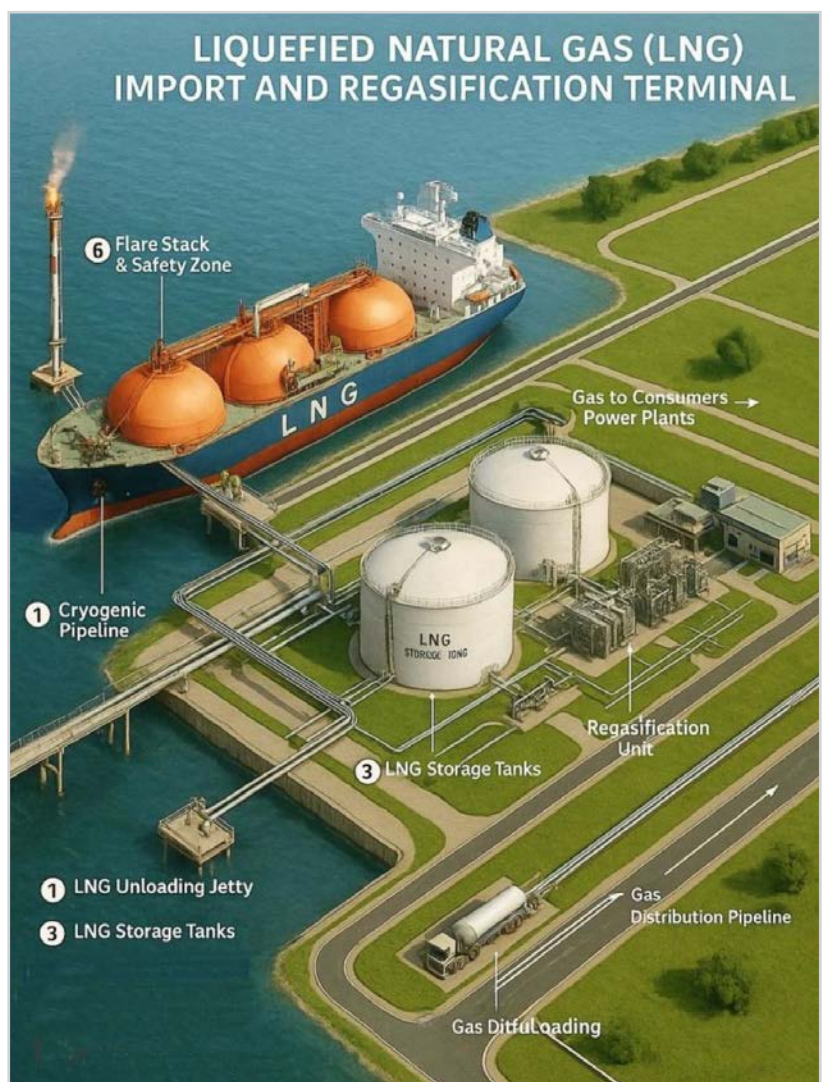
Figure 6: Liquefied Natural Gas (LNG) Import and Regasification Terminal Source: Commodity Trading Club
