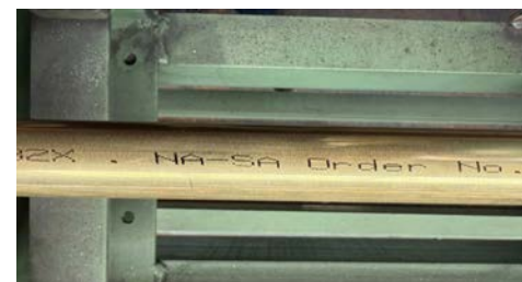
Fig. 5 Order and heat identification marked continuously along each tube length.
