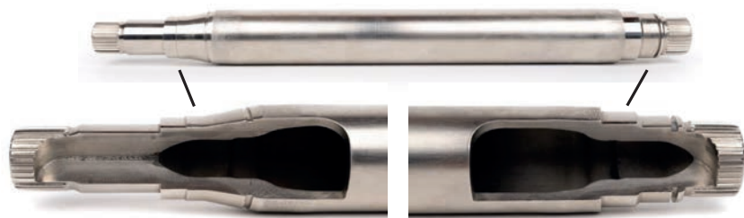
Fig. 3: Hollow drive shaft made from tube – realized component
