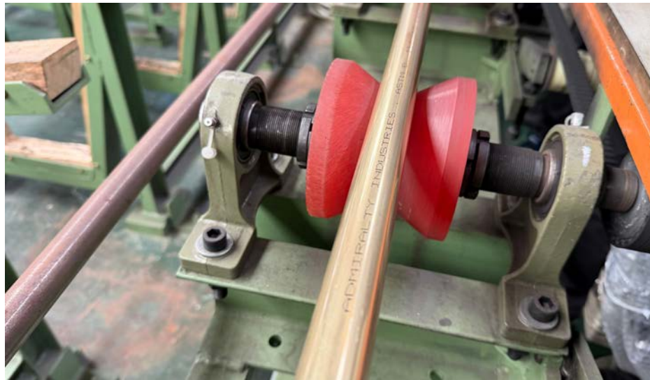
Fig. 2 Continuous marking applied in production — manufacturer, material specification and order reference — supporting traceability to individual tube level.
