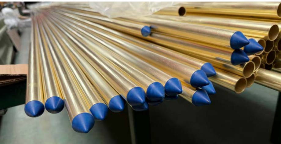
Fig. 1 Admiralty Brass condenser tubes to ASTM B111 UNS C44300, 25.40 mm OD × 1.24 mm minimum wall, end-capped following final inspection.
